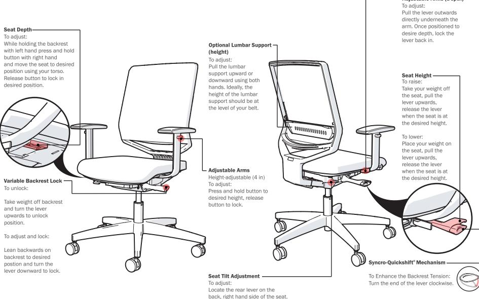
Rotate lever up or down to adjust the tilt.
